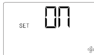
Fig.4.5-6 Ventilation function is on
